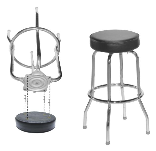
Remove screws from the upholstered seat using a #3 Phillips screwdriver. Rotate the swivel plate to the open position (as seen in diagram). Align swivel holes with the upholstered seat holes. Place one screw in each hole and tighten securely using a #3 Phillips screwdriver.
