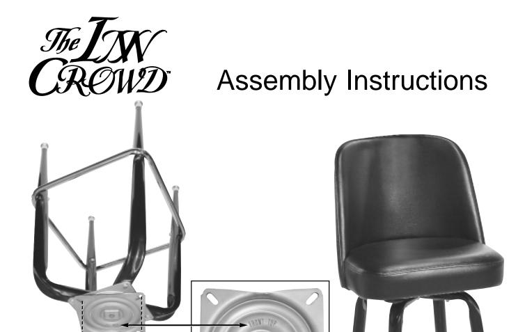
Remove screws from the upholstered seat using a #3 Phillips screwdriver. Rotate the swivel plate to the open position (as seen in diagram). Position the front of the bucket and the swivel plate so the words "FRONT-TOP" face the front of the bucket (see diagram of swivel plate). Align swivel holes with the upholstered seat holes. Place one screw in each hole and tighten securely using a #3 Phillips screwdriver.
